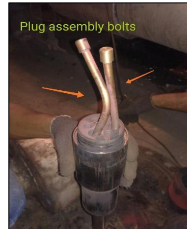
Upgradation of BFP RC valve trim set from single stage to multistage
