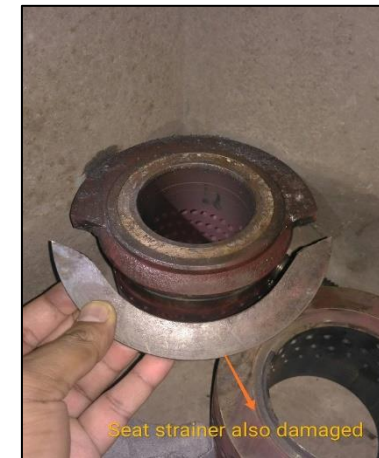
Upgradation of BFP RC valve trim set from single stage to multistage
